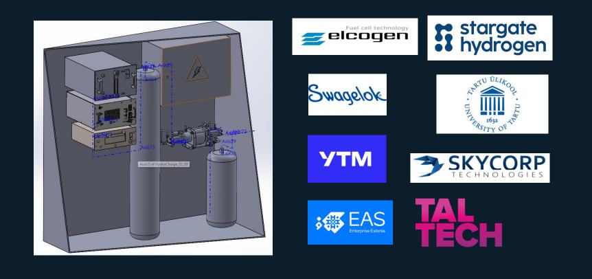
HydroSave is an energy storage project that utilizes metal hydride technology, creating a hydrogen storage system that is denser than liquid hydrogen and safer than lithium-ion batteries, suitable for defense applications, emergency energy storage, and seasonal energy storage.
